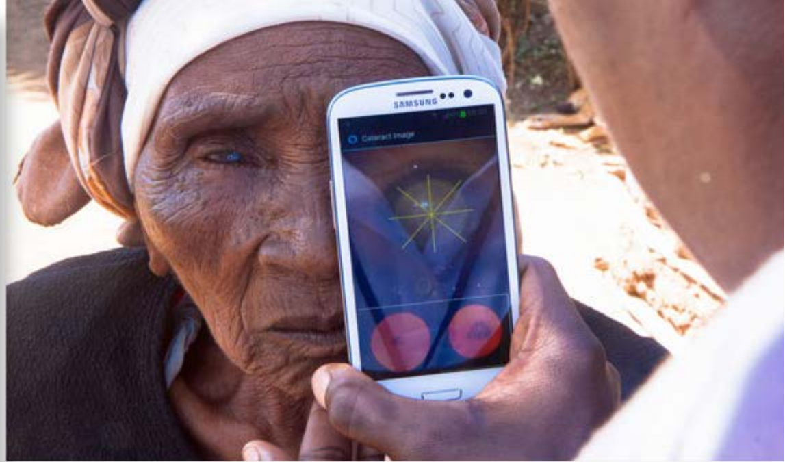
A woman from Nakuru, Kenya, having a cataract scan with the Peek smartphone tool. This portable eye testing kit can diagnose eye problems in remote areas, where access to clinics is limited. ©Peek
