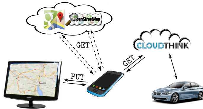
Figure 3-3: Semantic metadata allows flexible integration of CloudThink API data into local and remote web services. Here, a user requests a map with the location of their vehicle. A reasoner finds the appropriate requests to reach this goal and executes them. Figure ©2015 IEEE.
