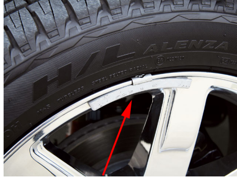
Figure 4-2: Wheel weights are used to balance automotive wheel and tire assemblies to provide a smooth ride and enhanced traction.
