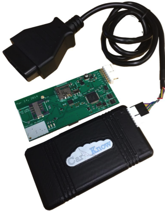
Figure 3-2: CarKnow's V8 Carduino device which connects vehicle CAN networks to the CloudThink API. Figure ©2015 Taylor & Francis.
