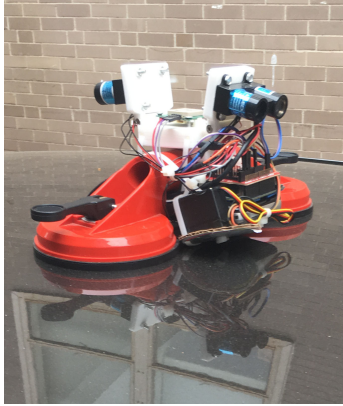
Figure 2-24: LidarBro V1, a self-contained GPS and LIDAR logging unit.
