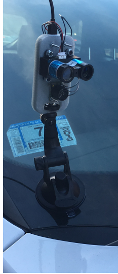
Figure 2-25: LidarBro V3, featuring SONAR and RADAR for redundant front distance sensing, which made use of separate Bluetooth-enabled GPS and OBD interface devices.
