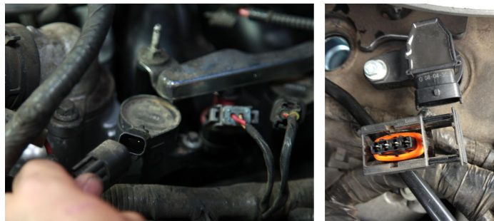
Figure 4-34: The supply to the ignition coil pack was disconnected in order to induce a complete misfire on individual cylinders.
