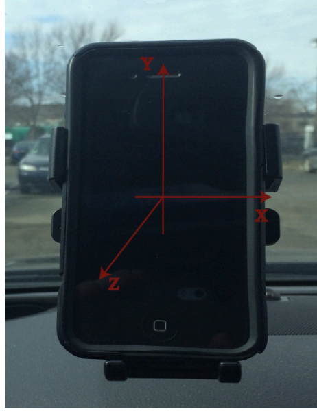
Figure 4-3: iPhone mounted in vertical orientation. The accelerometer directions are labeled. Figure ©2015 ASME.
