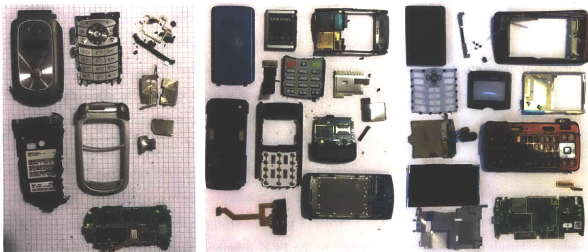
Figure 17. Dismantled mobile phones from batches 1, 2, and 3 (a. Motorola V325i H/W, 2005; b. Samsung SGH-A777, 2008; c. LG VX9200M, 2009)
