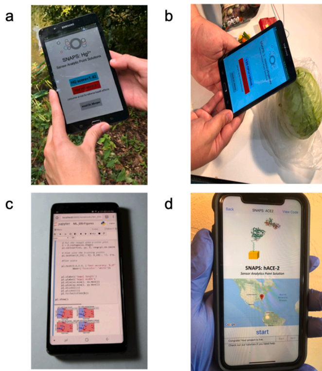
Fig. 12. Examples of SNAPS on-site sensing with embedded data analytics and decision support. a) Electrochemical aptasensor for detection of heavy metals in drinking water; reprinted from McLamore et al. (2019) with permission from © MDPI. b) Impedimetric aptasensor for measuring Listeria spp. in fresh produce samples; reprinted from McLamore et al. (2019) with permission from © MDPI. c) Smartphone machine learning analytics for sample classification in small protein sensing; reprinted from Rong et al. (2018) with permission from © Royal Society of Chemistry. d) Impedimetric biosensor for measuring SARS-CoV-2 on surfaces using the human receptor ACE-2; reprinted from Datta et al. (2020) with permission from © MIT Libraries.
