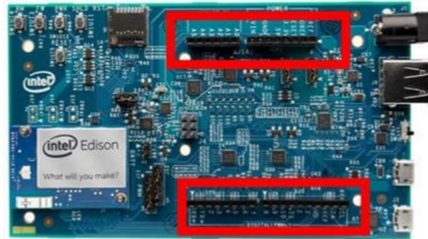
General Purpose In and Out – GPIO CPU, Memory (16 GB), WiFi, Bluetooth
