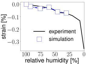
Upper: A depiction of the scheme proposed in this work to calculate the capillary forces in the pore structure. The C-S-H nano-particles (the main binding component of cement paste) are shown in maroon, tessellation cells are shown by blue-green columns. Inset showing water density distribution on the cell surfaces. Lower: cement paste first drying shrinkage strain curve.
