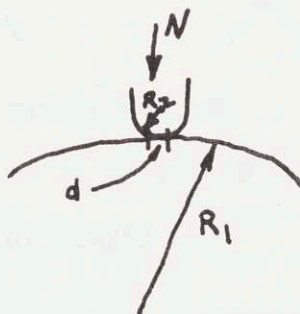
FIGURE 5. CONTACT BETWEEN ELASTIC SOLIDS
