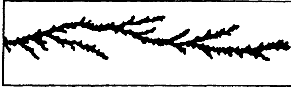
Typical viscous fingers created by water advancing into a linear Hele Shaw cell filled with a polymer solution (scleroglucan).
