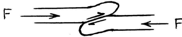
Figure 10. Situation from which weld stresses may be determined.
