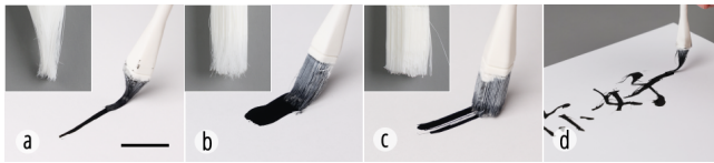
Figure 21: 3D Printed Brushes: (a-c) Brushes with varying stiffness; (d) Writing with a 3D printed brush. Scale Bar: 20 mm.
