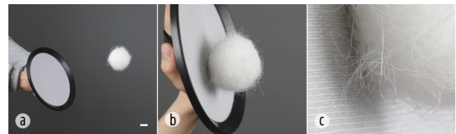
Figure 24: A 3D-printed velcro ball: (a) Throwing the velcro ball; (b) Catch the ball with velcro; (c) The detail of the ball. Scale Bar: 20 mm.
