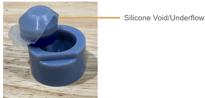
Figure 4. Prior cavity mold design, where silicone was poured after the poppet head was installed, which led to an air bubble causing a void/underflow defect.
