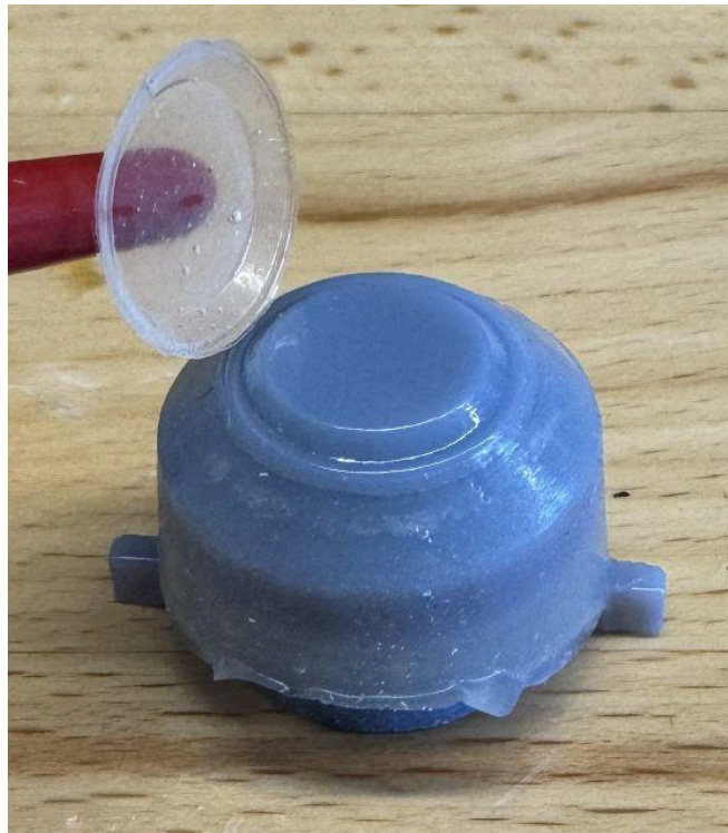
Figure 9: 0.5 mm thick ridged poppet head with silicone sheared off after high compression loads. Same effect occurred with 1 mm thick tapered poppet heads.
