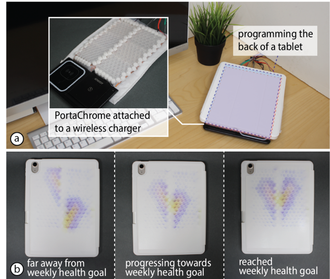
Figure 15: (a) PortaChrome can be attached to a wireless tablet charger and allows the back of the tablet to be reprogrammed while it is charging. (b) The back of this tablet case is reprogrammed to inform the user about their progress toward their weekly workout challenge.
