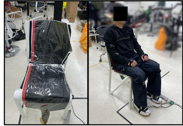
Figure 1: Hardware setup and data collection process. The left image shows the custom, high-density piezoresistive pressure sensing seat. The right image depicts a participant wearing the Perception Neuron Studio motion capture system, which provides the ground truth for three-dimensional skeleton data.
