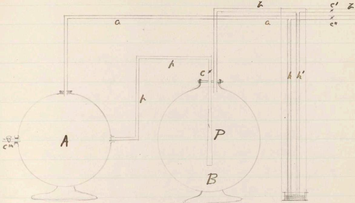
measure the pressures in the globes. In the globe B is placed a stopped lead organ pipe and this is connected by means of the tube h with the globe A; cocks are placed at e, c', c''' and c''''.
