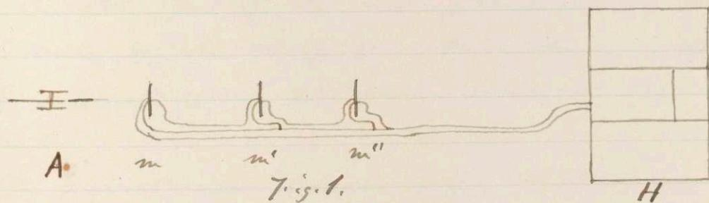
At A. (Fig. 1) was the gun, at  $m$ ,  $m'$ ,  $m''$  the membranes, and at H the house in which was a battery room B and an instrument room in which were mounted on stone piers a Schultz and a Le Boulay's chronograph. The meteorological instruments too were placed in this room.
