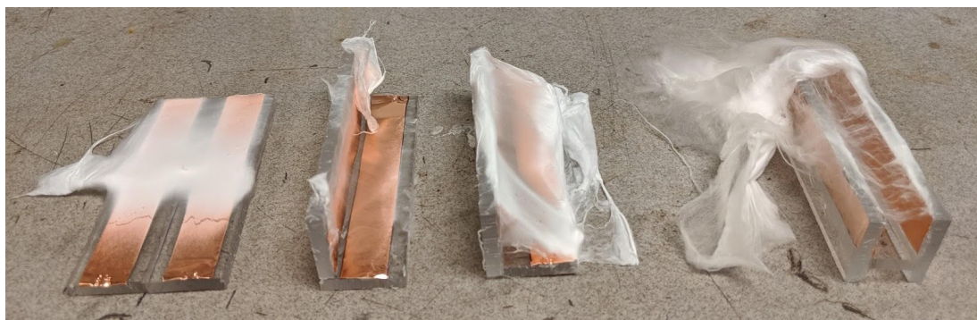
Fig. 6 Electrospun gelatin scaffolds on two separated plates show that fibers can be visibly aligned by varying the angle between the plates.
