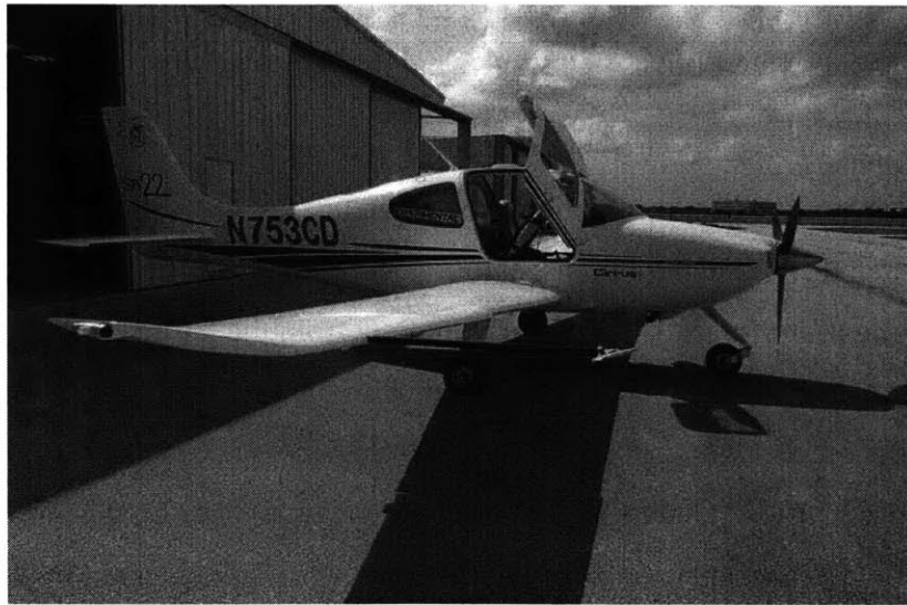
Figure 13: Experimental Cirrus SR22 N753CD used for test flights, with angle of attack vane mounted on the boom of a modified wingtip
