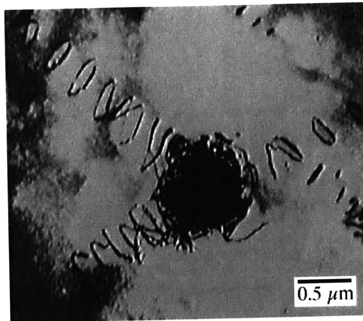
FIGURE 2. Tangled and free dislocation loops formed by precipitation of niobium hydrides in niobium. From MAKENAS AND BIRNBAUM 1980.
