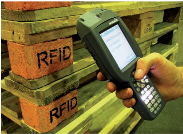
Figure 40. The use of RFID will become more common in transport units. Here RFID-tags installed to pallets are read. Source: Vilant Systems Oy
