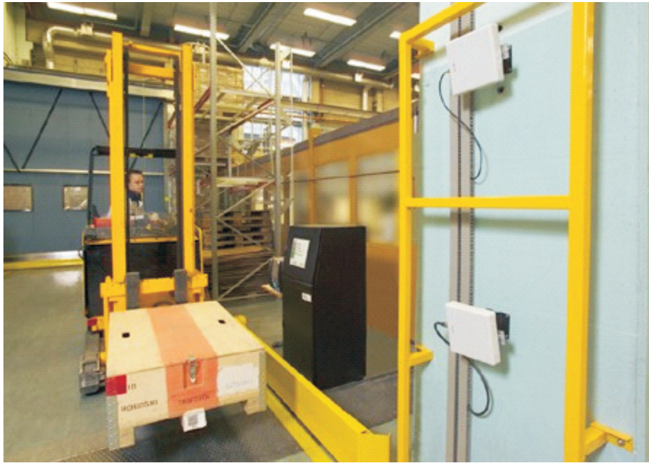
Figure 15. RFID tags are read when components are delivered to factory.
