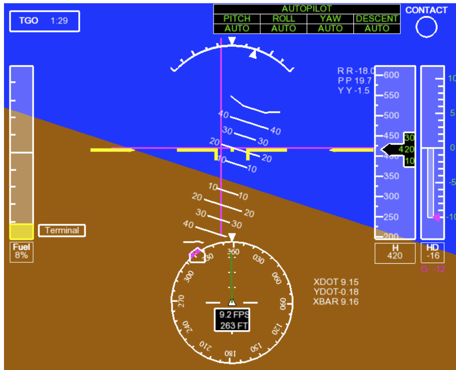
Figure 7.2: Primary Flight Display
