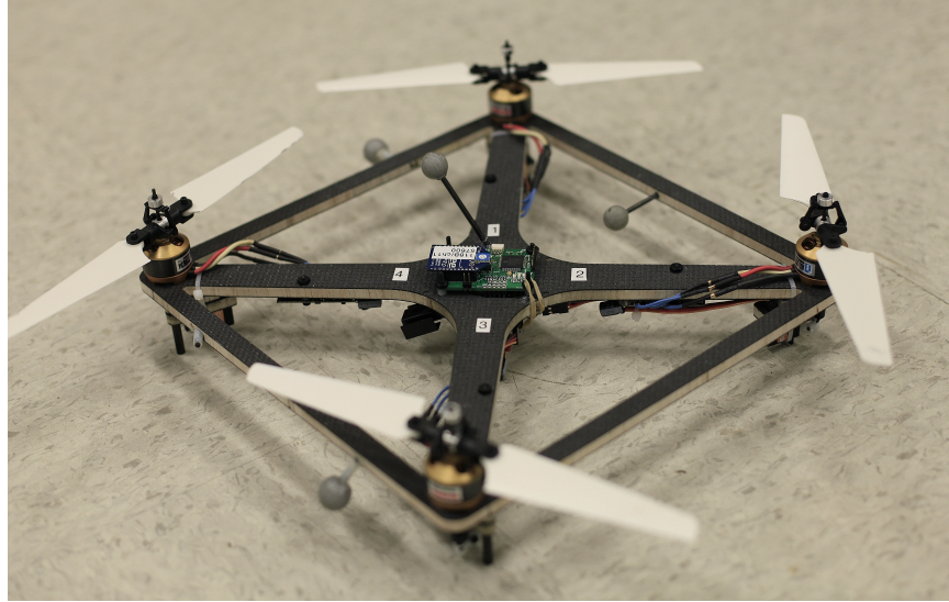
Figure 4-1: Variable-pitch quadrotor designed at the Aerospace Controls Lab. The servos that actuate the variable-pitch propellers are visible under each of the motors. The quadrotor measures 0.35 m across.
