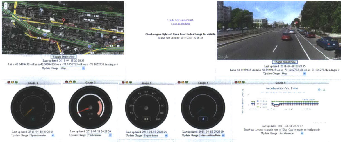
Figure 23: Teen tracker software displays a reconfigurable virtual dashboard Find my car: This software locates the last location the vehicle was operated and renders this point on a map.
